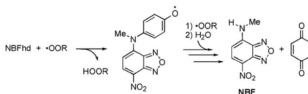
**Scheme 2** Proposed mechanism of reaction of the NBFhd sensor with peroxy radicals.
