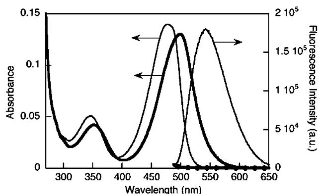
Fig. 1 Absorption (left) and fluorescence (right) spectra of a  $5 \times 10^{-6}\ M$  solution of NBF (thin line) and NBFhd (thick line) in phosphate buffer solution (PBS) at pH 7.4. The excitation wavelength was set at 468 nm and fluorescence spectra (right axis) for unexposed samples include a few identifier points (●).
